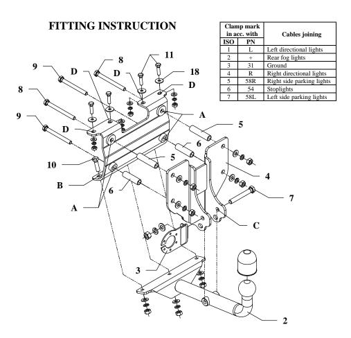
This towing hitch is designed to assembly in following cars: **OPEL ASTRA (F) Caravan ESTATE,** produced since 09.1991 till 2002, catalogue no. **E19** and is prepared to tow trailers max total weight **1500 kg** and max vertical mass **75 kg**.
